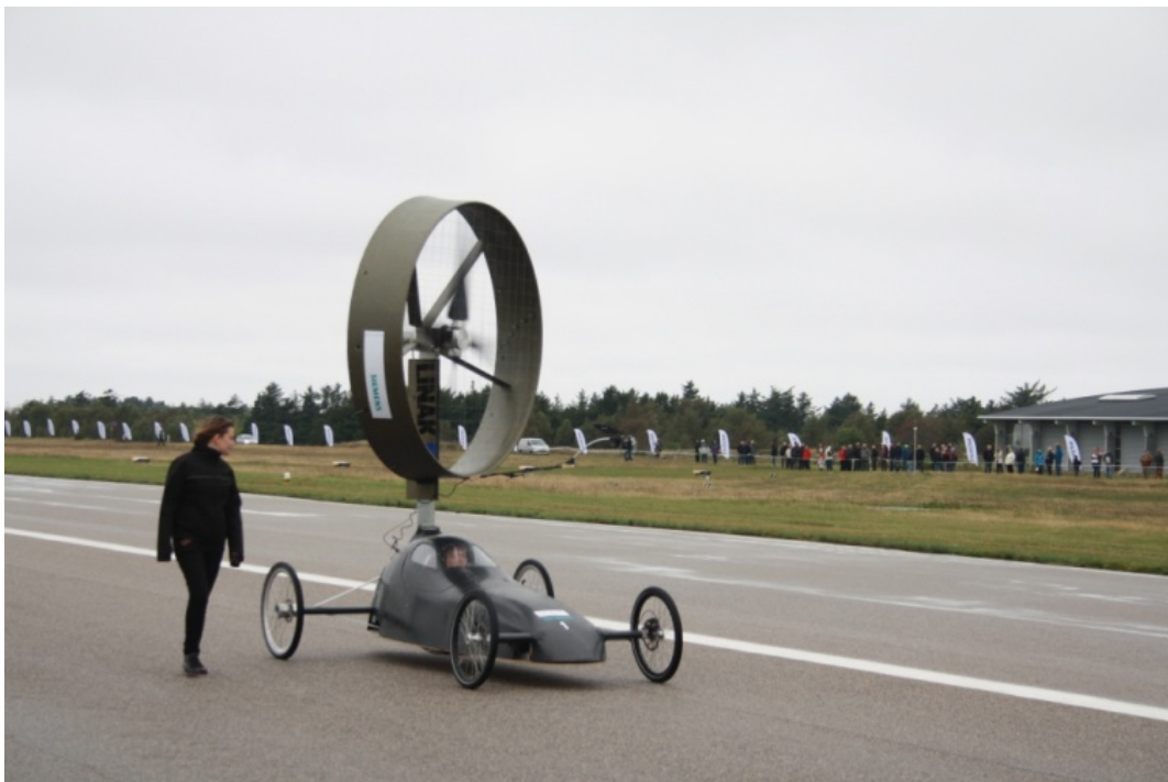
Figure 6 Technical University of Denmark. DTU1, winDTUrbineracer 1
